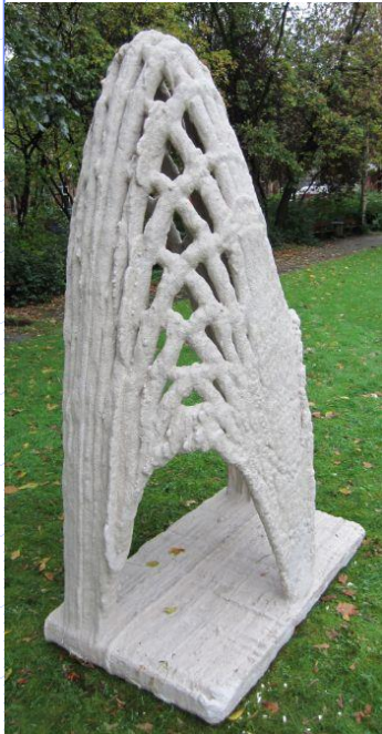
Pavilion (concrete 3D print, D-shape)
