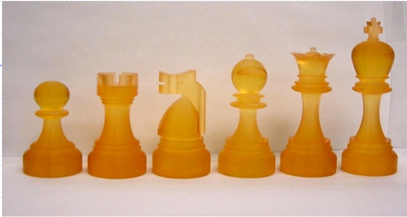
Chess pieces (resin & stereolithography)
